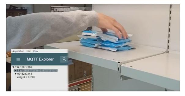
The picture belongs to the test that we made in order to verify the correct workability of the reader. After checking that the shelf where we are going to place the products is straightened correctly, we use different samples. The test starts just with one product and, later, more products will be added. MIMEX cloud shows a correct correlation between the number of placed products and the weight detected, even if we place different kinds of products (in
